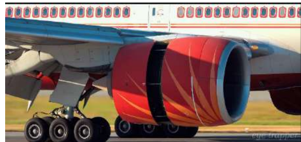
Figure 9: B777 cascade type reverse thrust.
