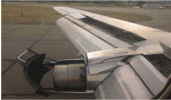
Figure 11: B737-200 Target type reverser.
