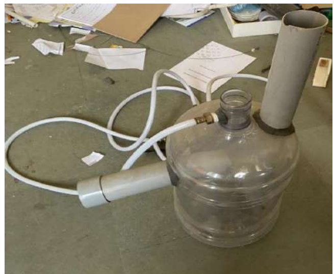
Figure 6.3. Physical setup of digester
