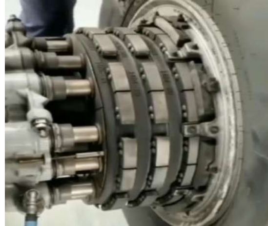
Figure 12: Hydraulic brake assembly of A320.
