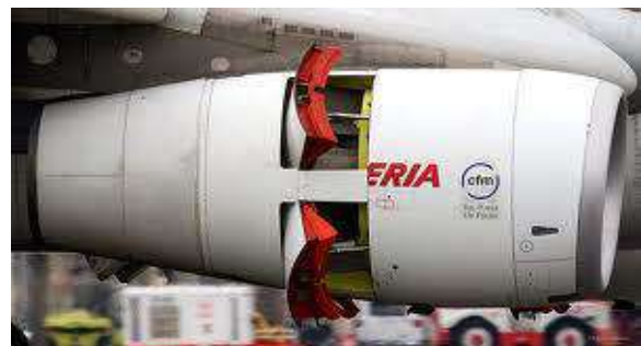
Figure 10: A330 clamshell reverse thrust.
