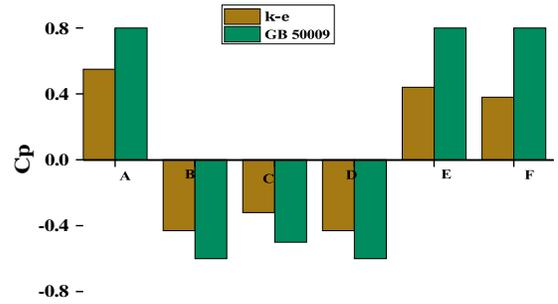
Pressure Coefficient on Mean Cp at model-A
