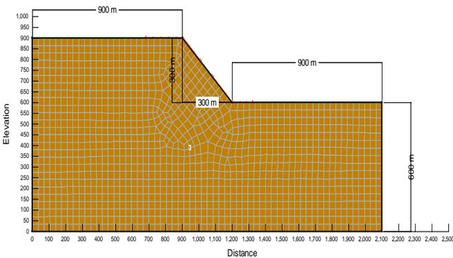
**Fig. 5: Geometry of unsaturated slope before rainfall**
