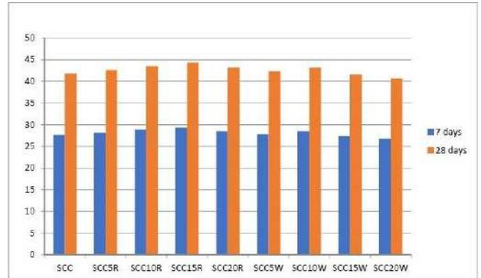
Fig 4.4 Compressive strength variation with different proportions of RHA or WSA in SCC
