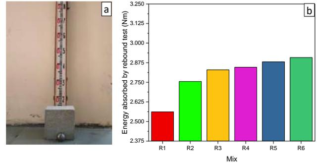
Fig. 6(a) Testing setup of Impact resistance by rebound test (b) Impact energy absorbed by the rebound of standard and RuC mixes
