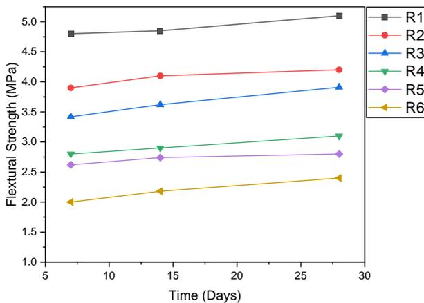
Fig. 5 Flexural strength of standard concrete and RuC
