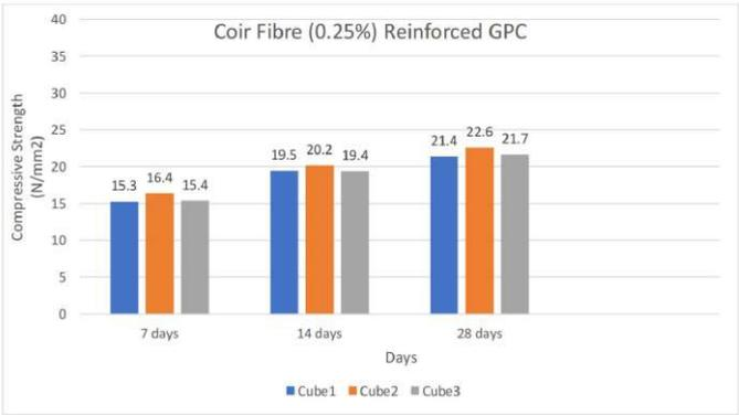
Fig 3.10 Graph of Coir Fibre(0.25%) Reinforced GPC
