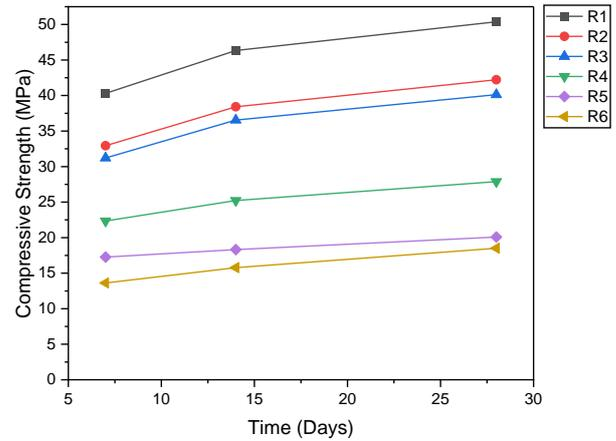
Fig. 3 Compressive strength of standard concrete and RuC
