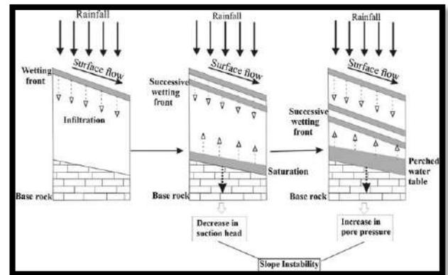
**Fig. 11: A sequential schema of shallow landslide initiation [19]**
