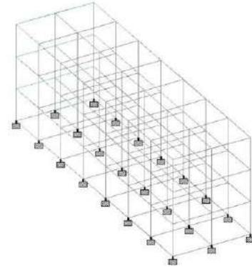
Fig. 3. Short span (6m) model on STAAD Pro for Static Analysis
