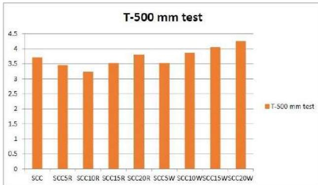
Fig 4.2 - Variation in the T-500 mm flow time at different % of RHA or WSA in SCC
