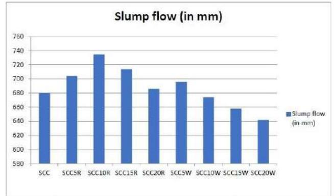
Fig 4.1 Variation in the slump flow at different proportions of RHA and WSA in SCC
