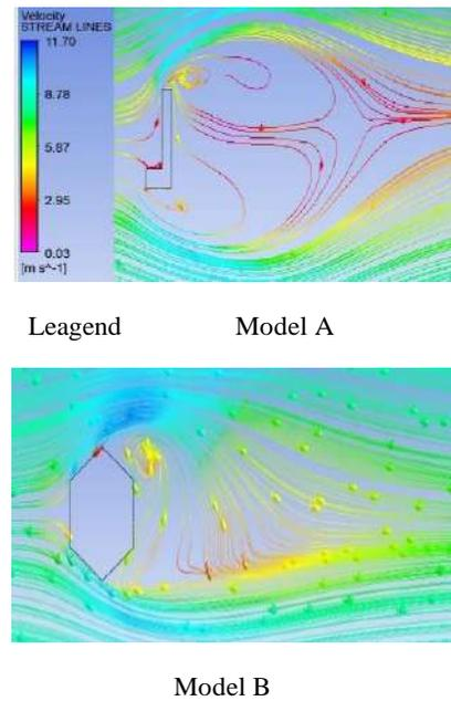
**Fig. 7** wind flow patterns around the building model in plan
