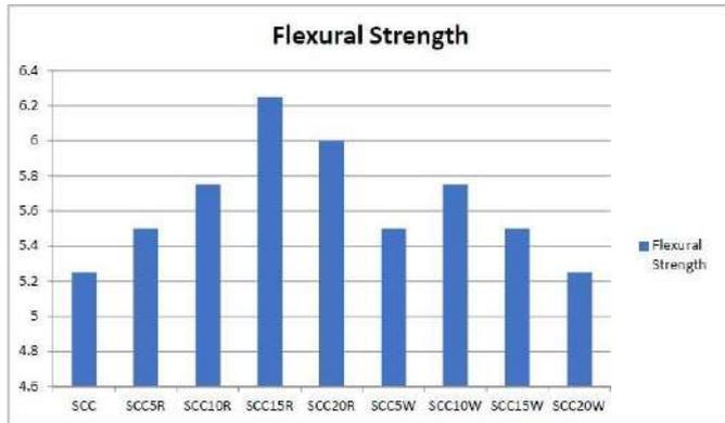
Fig 4.6 Variation in flexural strength with different proportions of RHA or WSA in SCC
