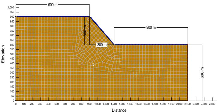
**Fig. 6: Geometry of slope with rainfall**
