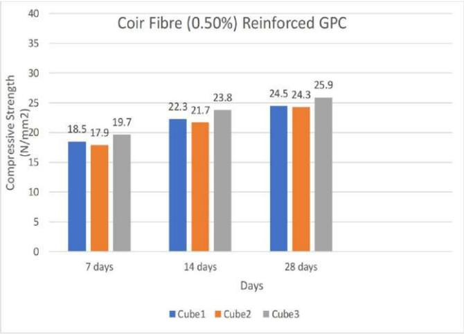
Fig 3.9 Graph of Coir Fibre(0.50%) Reinforced GPC
