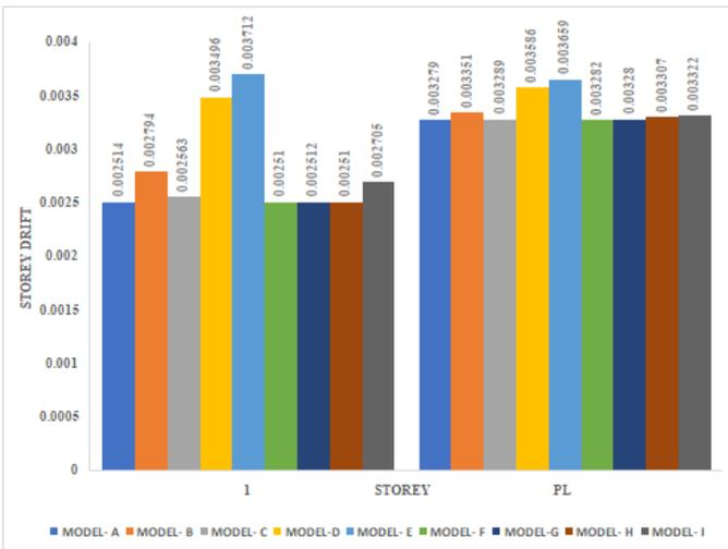
Fig. 4. Storey Drift in Y Direction
