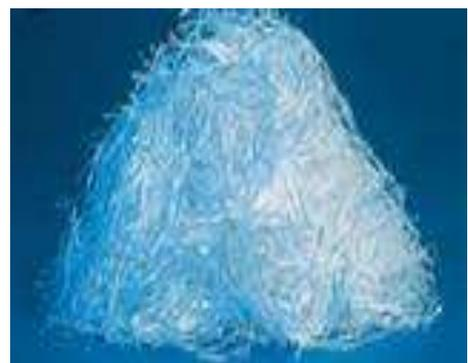
**Figure 6: Milled Steel Fiber**
