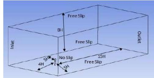
Fig.2 Computational Domain dimensions and boundary condition
