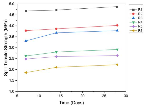
Fig. 4 Split tensile strength of standard concrete and RuC
