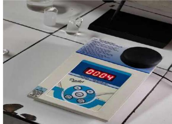
Fig.5 Nephelometer Turbidity Test
