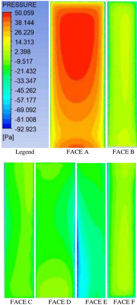
**Fig.6** Pressure Contour on Building Model -B
