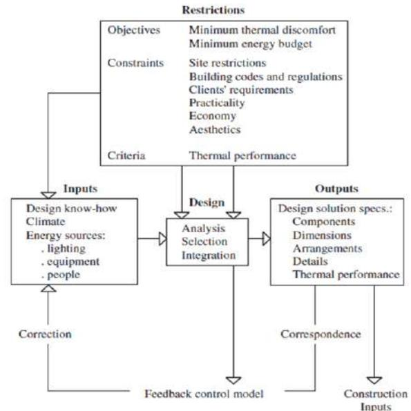
Figure 2. Structure of building thermal design optimization process.
