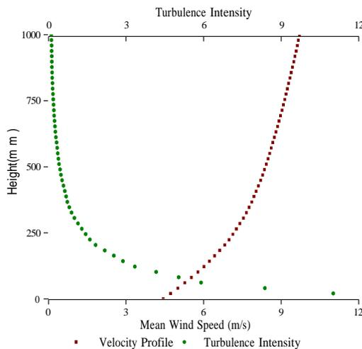
**Fig.4** Velocity profile and Turbulent Intensity profile
